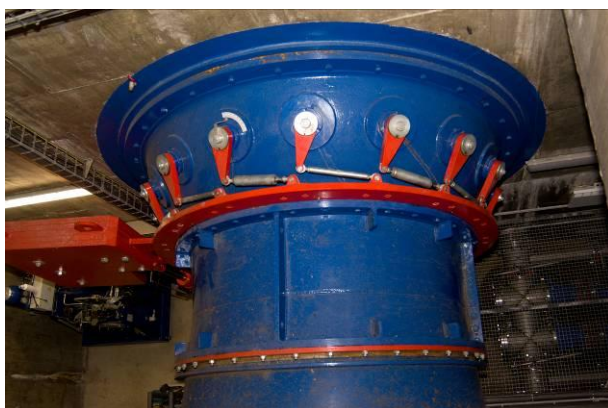
Turbína : Kaplanova PIT turbína, PT = 848 kW, 200 ot/min
